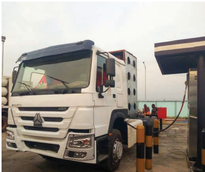
REDUCING FUEL CONSUMPTION BY CONVERTING TRUCKS TO CNG AT IMPALA IN NIGERIA
